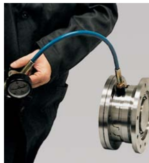
6 Relief pressure in pump and disconnect the same. Insert sealing plug into injector connection.
