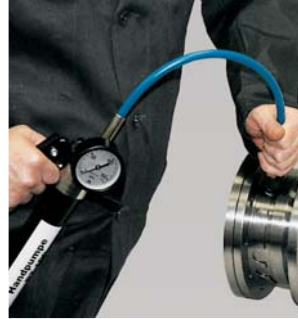
4 Connect pump, loosen shear tube by 1/4 turn.
